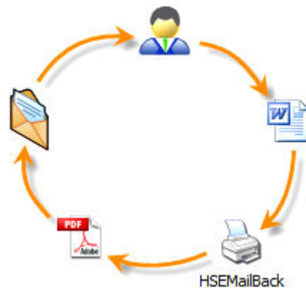
FIGURE 24 - a user creates a document, prints it with a mailback printer, which converts it to PDF and sends it via e-mail back to the user who printed the document.
